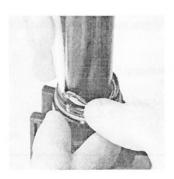
When installing the X-ring into the Collar Nut, be careful to work it in gradually using a blunt tool. It must be fully seated into the Collar Nut, or else the SSR will be over compressed when the Collar Nut is tightened and the benefits of the SSR will be diminished or lost.
