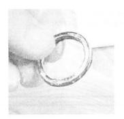
Apply only a thin film of P10L grease to the X-ring seal to aid in installation.
