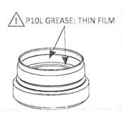
Successful installation of the SSR requires careful attention to the amount and location of grease applied, proper seating of the x-ring, and correct installation of the SSR itself.
